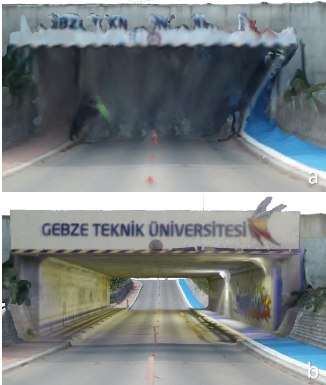
Figure 5. 3D model of the underground pass produced using RGB UAV dense cloud (a) and using the fusion of RGB UAV dense cloud and colored terrestrial laser scanner dense cloud (b)
