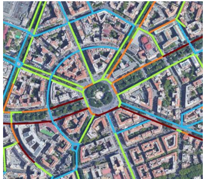
Figure 4. Rome, Square Mazzini. The processing highlights the total emissions g/h calculated from the traffic flow data
