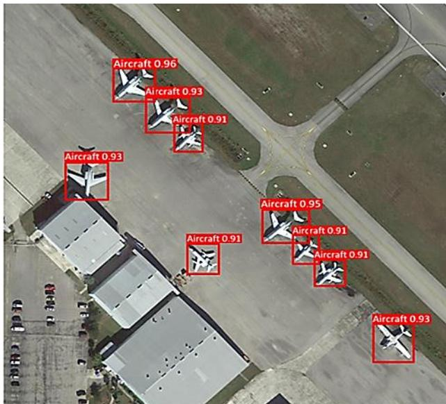
Figure 1. Detection previews from YOLOv7 Architecture
