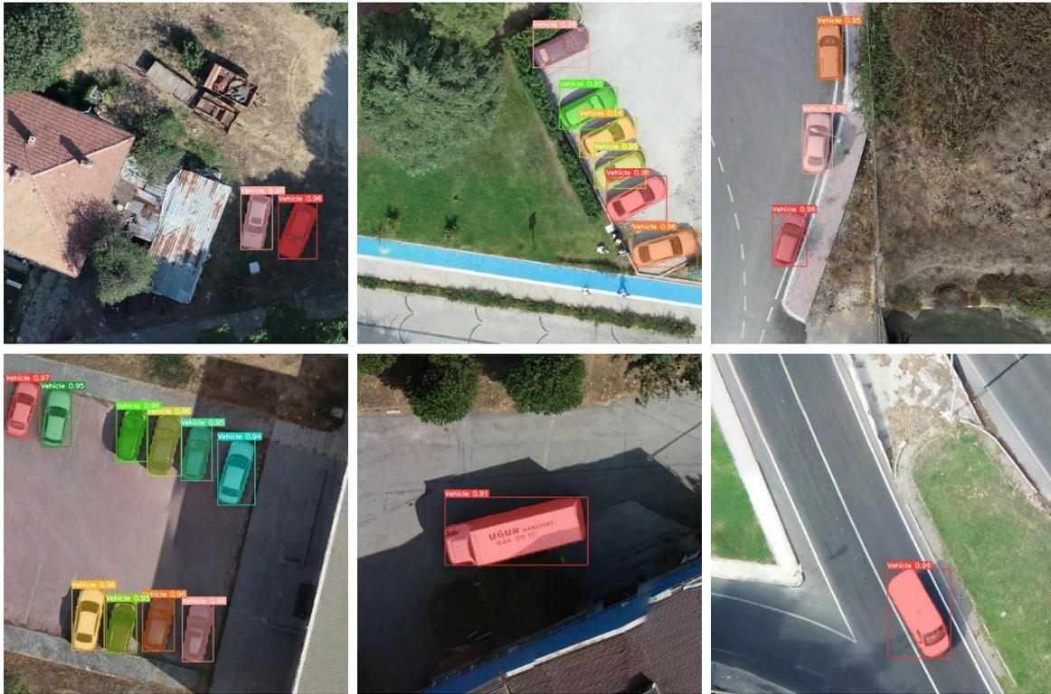
**Figure 5.** Examples of vehicle detection and instance segmentation results of the YOLOv7 model
