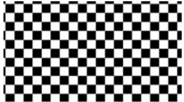
Figure 2. Agisoft Lens software calibration chessboard
