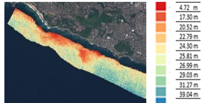
Figure 4. ln (blue) / ln (green) forecast bathymetry map
