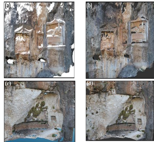
Figure 2. (a), (c) Point cloud obtained by TLS method (b), (d) 3D model.
