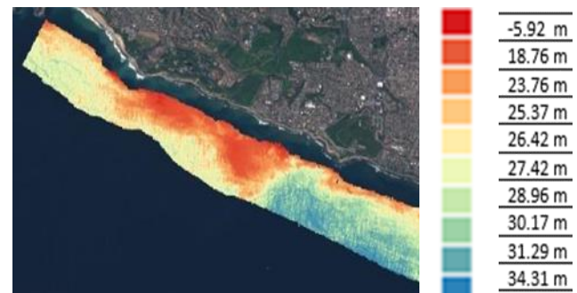
Figure 5. ln (green) + ln (blue) + ln (red) forecast bathymetry map
