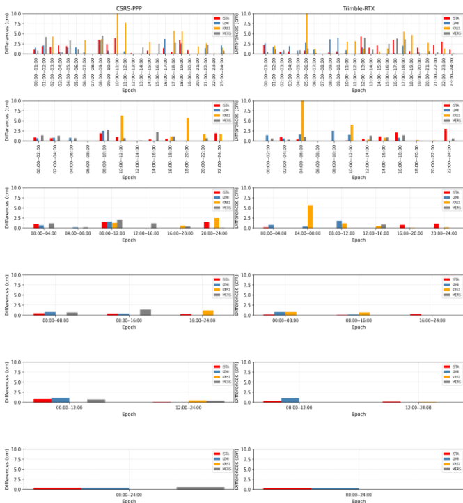
Figure 4. Height differences between known-coordinates and online services for GPS only constellation ( left ; CSRS-PPP, right : Trimble RTX-PP).
