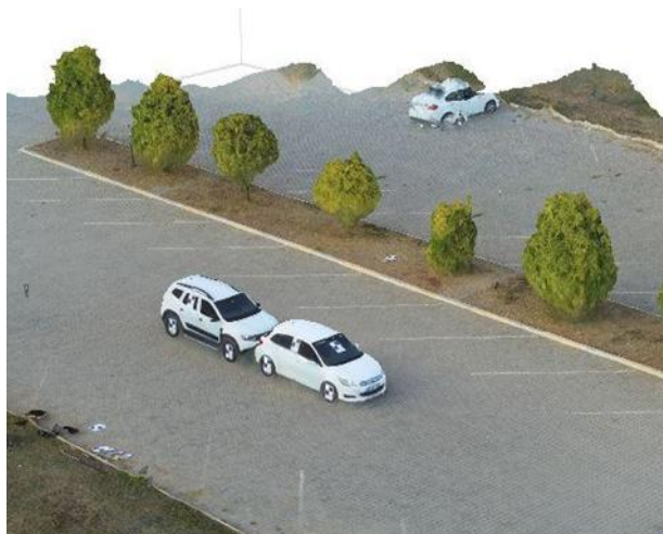
Figure 5. Textured model obtained by the use of UAV images
